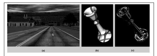
Figure 3. (a) A scene with a number of textures mapped onto primitives. (b) Contouring achieved with texture mapping and a texture coordinate generation function. (c) Reflectance mapping with a texture coordinate generation function.
