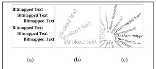
Figure 5. (a) Bitmap example. (b) Stroke font example. (c) Texture mapped font example.
