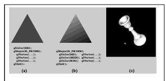
Figure 2. (a) A uniformly colored triangle. (b) A Gouraud shaded triangle. (c) A scene consisting of many lit, shaded polygons.
