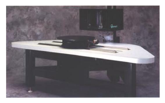
Figure 1.5: A photograph of the Cyberware Model MS 3030 optical triangulation scanner used for acquiring range images in this thesis.
