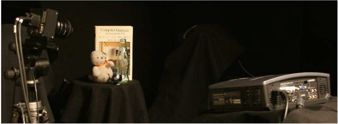
Figure 3.5: Setup for dual photography. A pattern loaded into projector on the right illuminates the scene and the camera on the left records the outgoing radiance. The camera used is a Basler A504kc (1280 × 1024 pixels) and the projector is a Mitsubishi X480U (1024 × 768 pixels). The setup is computer controlled, and we capture HDR images every 2.5 seconds.
