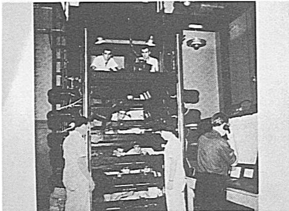
Figure 1a: The multiplane camera stand used by Walt Disney in his productions of the 1930's.
