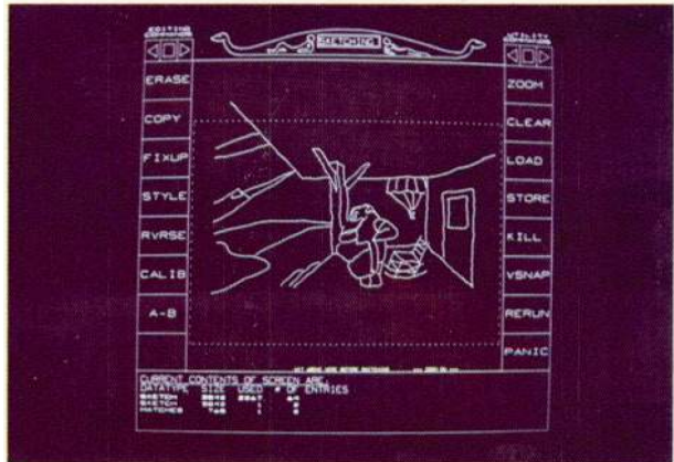
Figure 4b: Vector approximation of 4a for display on vector scope (allowing real-time manipulation).
