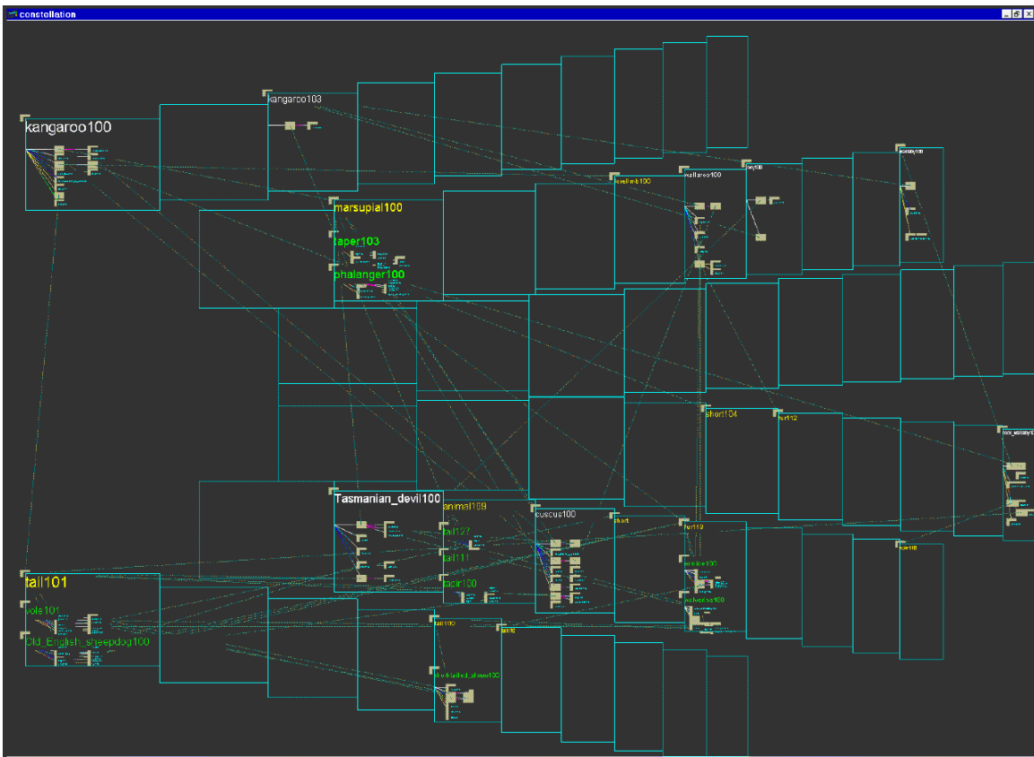
Figure 5.12: Early sparse layout. An earlier version of the software used only the base layout algorithm described in the previous sections, which is successful at encoding the plausibility spatially but results in a somewhat sparse layout with only about 20 legible words.
