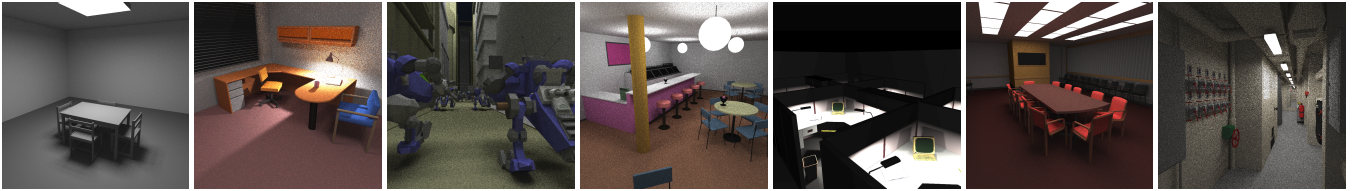
Figure 3: Test scenes used in our experiments. From left to right: erw6 (804 triangles, 1 quad light); office (34K, 2 quad lights, 1 sphere light); robots (72K, 1 quad light); soda shoppe (141K, 6 sphere lights); nrc-office (222K, 12 quad lights); conference (280K, 1 quad light); and cruiser (3.6M triangles, 1 quad light). All images are rendered with a two-bounce diffuse path tracer with 1 sample per light and 64 samples per pixel.
