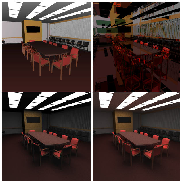
Figure 2: EyeLight shader (primary rays), perfectly specular reflections (2 bounces), soft shadows (16 samples per light), and path tracing (2 bounces, 1 sample per light) for the conference scene.
