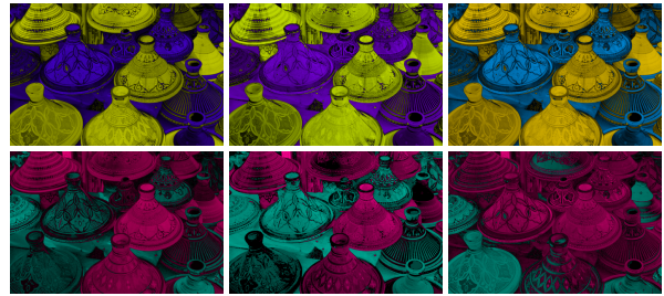
Figure 4: Visualization of the chroma channels for (left to right): YCC , l\alpha\beta , and CIE L*a*b* color spaces. Compared to our new oRGB space (Figure 1), these spaces do not have a true red-green channel.
