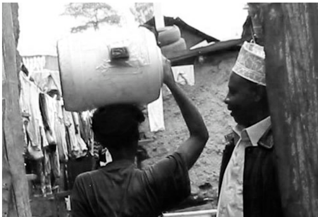
Figure 3. GPS unit attached to jerry can. Study participant is carrying jerry can of water weighing 20kg from a vendor's tap to her home.
