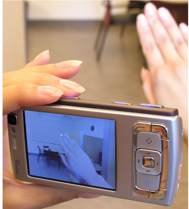
Figure 1: The user can control the pointer by simply moving his or her hand behind the phone.
