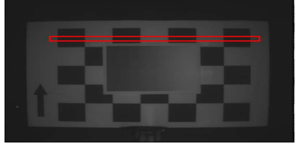
Figure 6: Test target. The region inside the red rectangle was used to evaluate depth. The mean calculated depth of each column under several different conditions is plotted in Figures 7 and 8.
