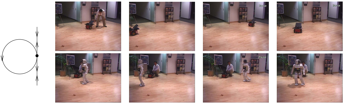
Fig. 10. Snapshots of a motion sequence using GOTO commands, executed on a Pioneer 2 (top row) and Honda's ASIMO (bottom row). The target path is shown on the left. The motion was coupled with pan and tilt actions for joint #1 (the head). We intentionally defined the pin-tilt joint of the camera on Pioneer 2 as joint #1. The client sent the same sequence without knowing the driver implementation.
