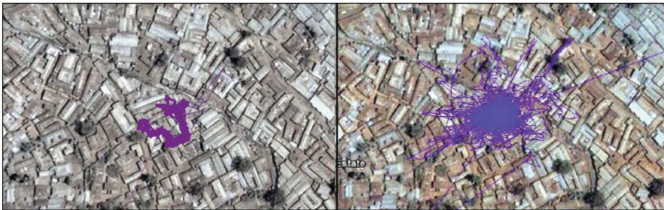
Figure 6. Noisy GPS readings (right). The magnitude of the noise is greater than the intended track recording distance (left).
